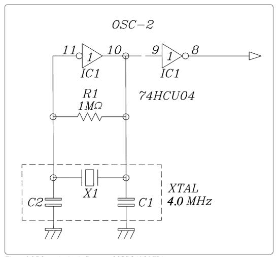
Figure 4.6 Schematic circuit diagram of OSC-2 (4.0 MHz)
